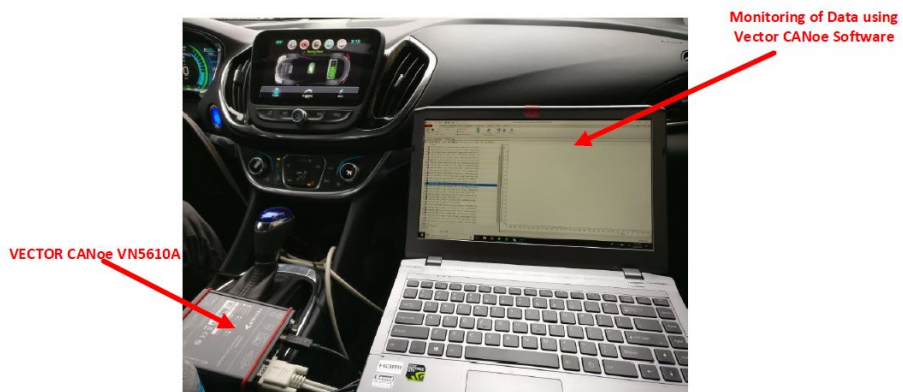
Figure 2.2: Data Acquisition using Vector CANoe VN5610A
